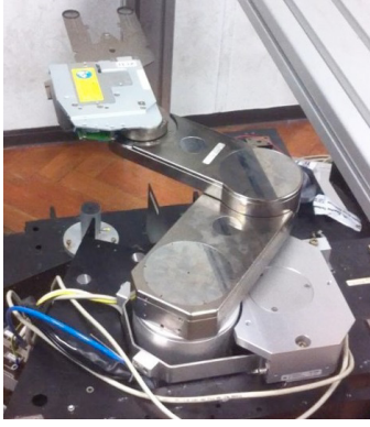
Fig. 1. Experimental SCARA robot. The object is normally positioned at the end of the wrist, with its center between the two black rubber rings.
