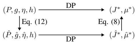
Fig. 2. Solving the original problem (P, g, \eta, h) in feature space M by lossless feature mapping \phi generating proxy problem (\hat{P}, \hat{g}, \hat{\eta}, h) with state space cardinality m < n . An optimal solution pair (\mu^*, J^*) is losslessly recovered from (\hat{\mu}^*, \hat{J}^*) .
