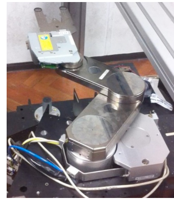
Fig. 8. Experimental SCARA robot. The object is normally positioned at the end of the wrist, with its center between the two black rubber rings.
