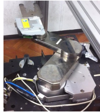
Fig. 8. Experimental SCARA robot. The object is normally positioned at the end of the wrist, with its center between the two black rubber rings.
