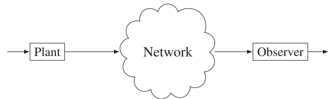
Fig. 1. Network-induced imperfections in the form of intermittent loss of plant output (see Section III).
