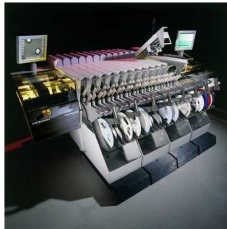
Fig. 1. Fast component mouter (courtesy of Assembleon)
