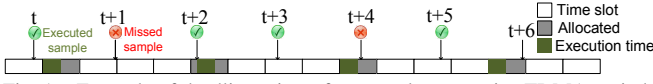
Fig. 1. Example of deadline misses for several consecutive TDMA periods where the second of four time slots is assigned to \lambda_C and e_C = \frac{1}{2}T_{TS} .
