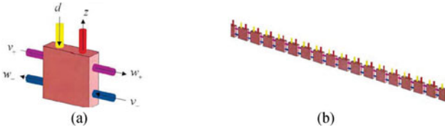
Fig. 1. Spatially invariant interconnected systems in one spatial dimension from [6]. (a) Basic building block. (b) Infinite interconnection.
